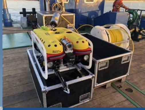
Cable depth of burial surveying using acoustic and ROV inspection techniques.
