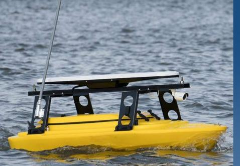
The Z-Boat 1800 remote hydrographic survey boat with Kongsberg GeoSwath 4R
