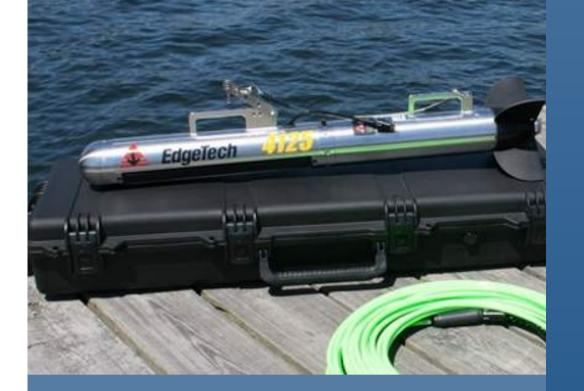
High-resolution seabed mapping using advanced mulitbeam echosounder and side scan sonar systems.
