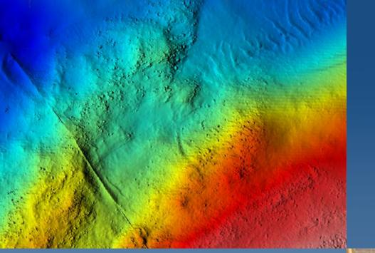
Ultra-high resolution multibeam bathymetry for scour monitoring, cable exposures and freespan identification.
