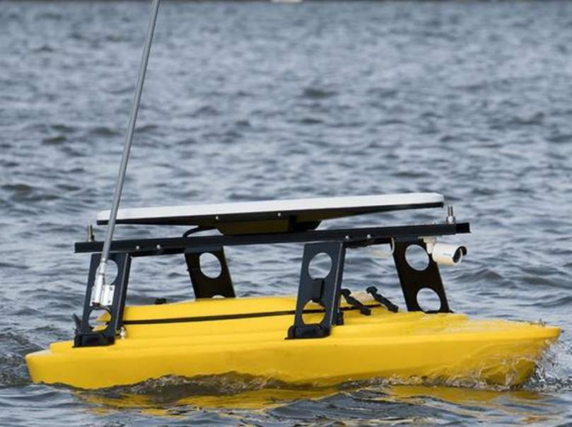
The Z-Boat 1800 remote hydrographic survey boat with Kongsberg GeoSwath 4R
